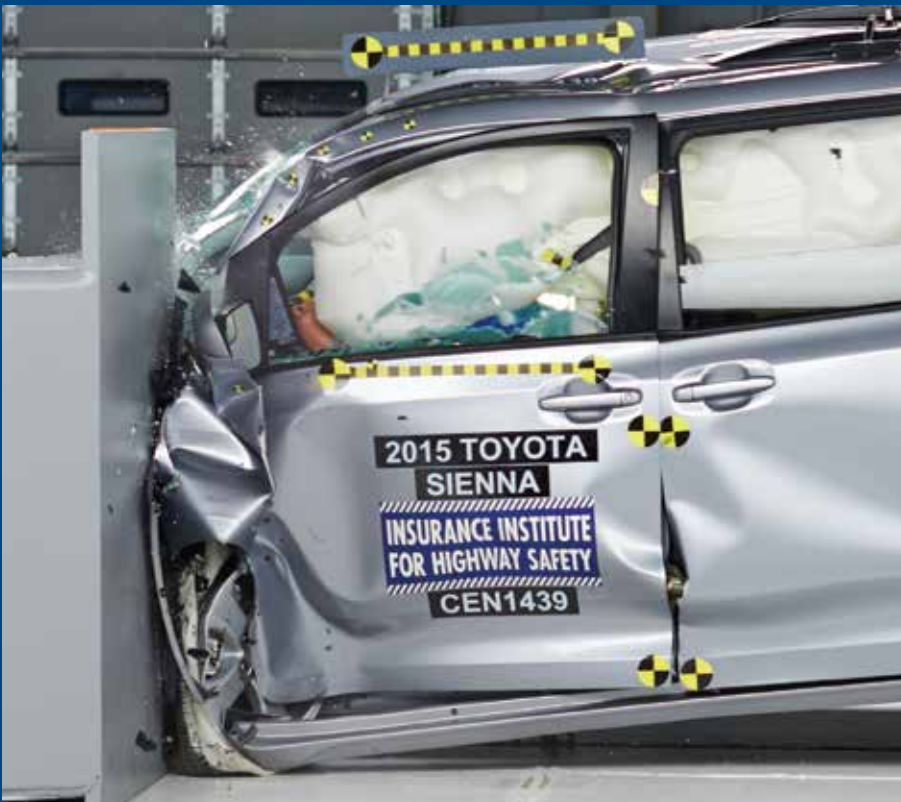
The door hinge pillar and instrument panel were pushed in 5½ inches during the test of the Toyota Sienna (left), but the minivan still managed an acceptable rating overall. Intrusion in the poor-rated Nissan Quest was much worse, reaching nearly 2 feet and completely trapping the dummy's left leg.
