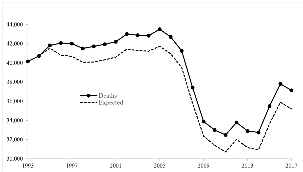
Figure 1. Traffic fatalities in the U.S., 1993–2017, and expected deaths if maximum speed limits had not increased.
