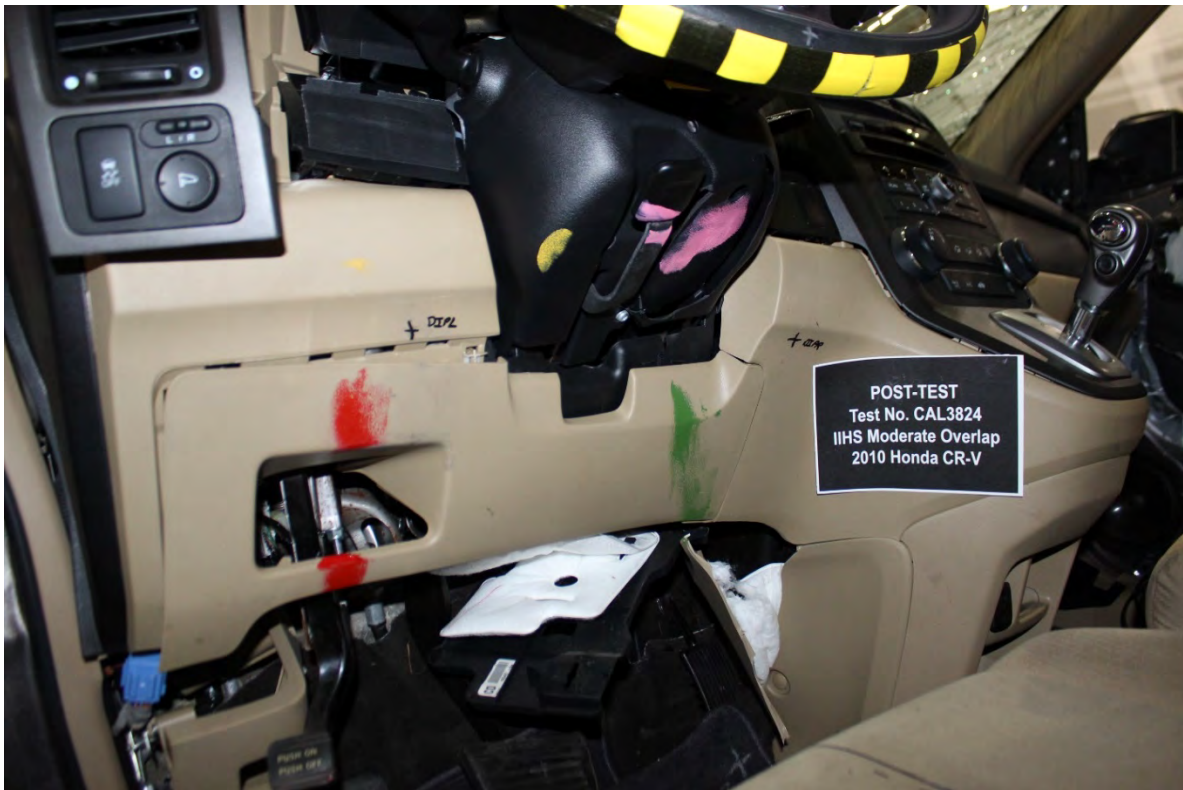
Vehicle intrusion and paint mark from dummy after displacing the dummy
