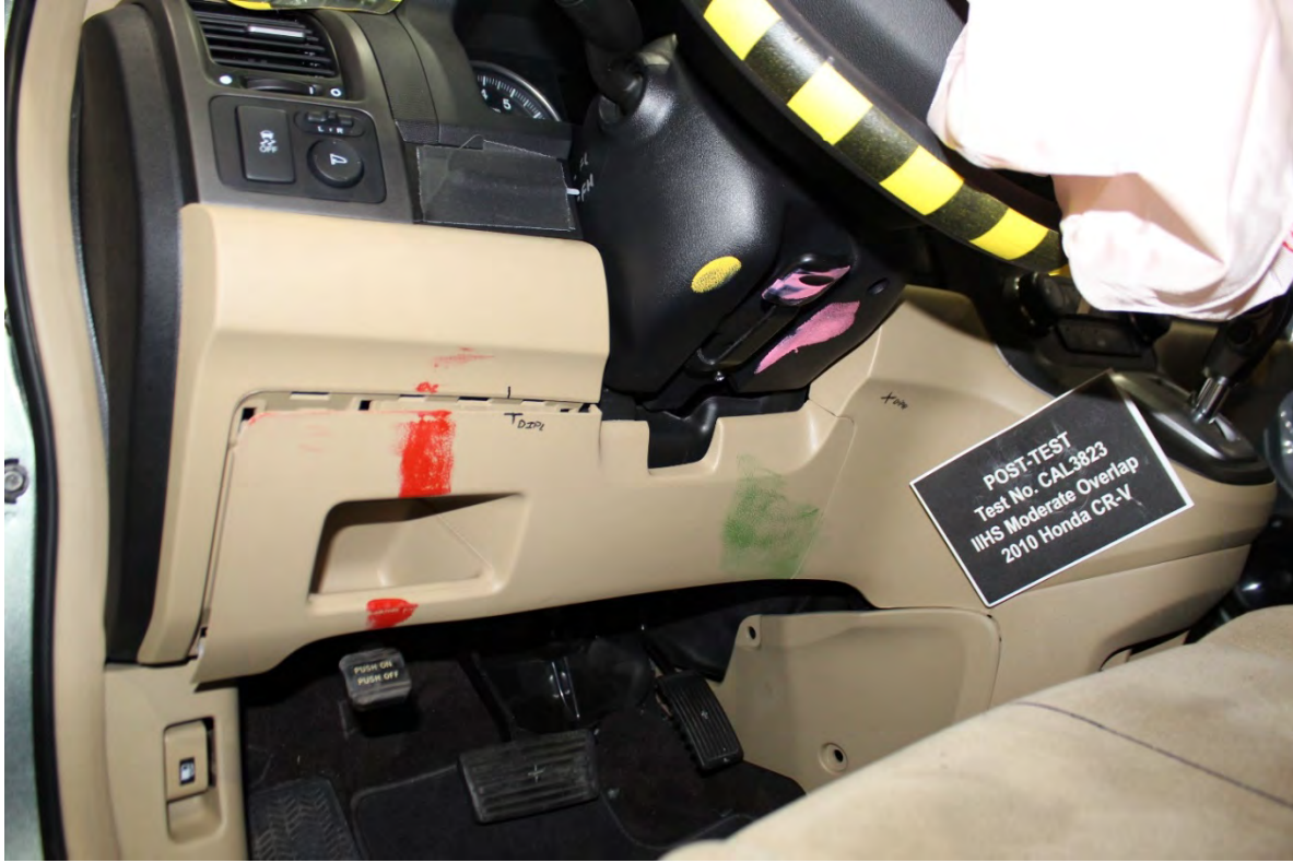
Footwell intrusion and paint mark from dummy's body
