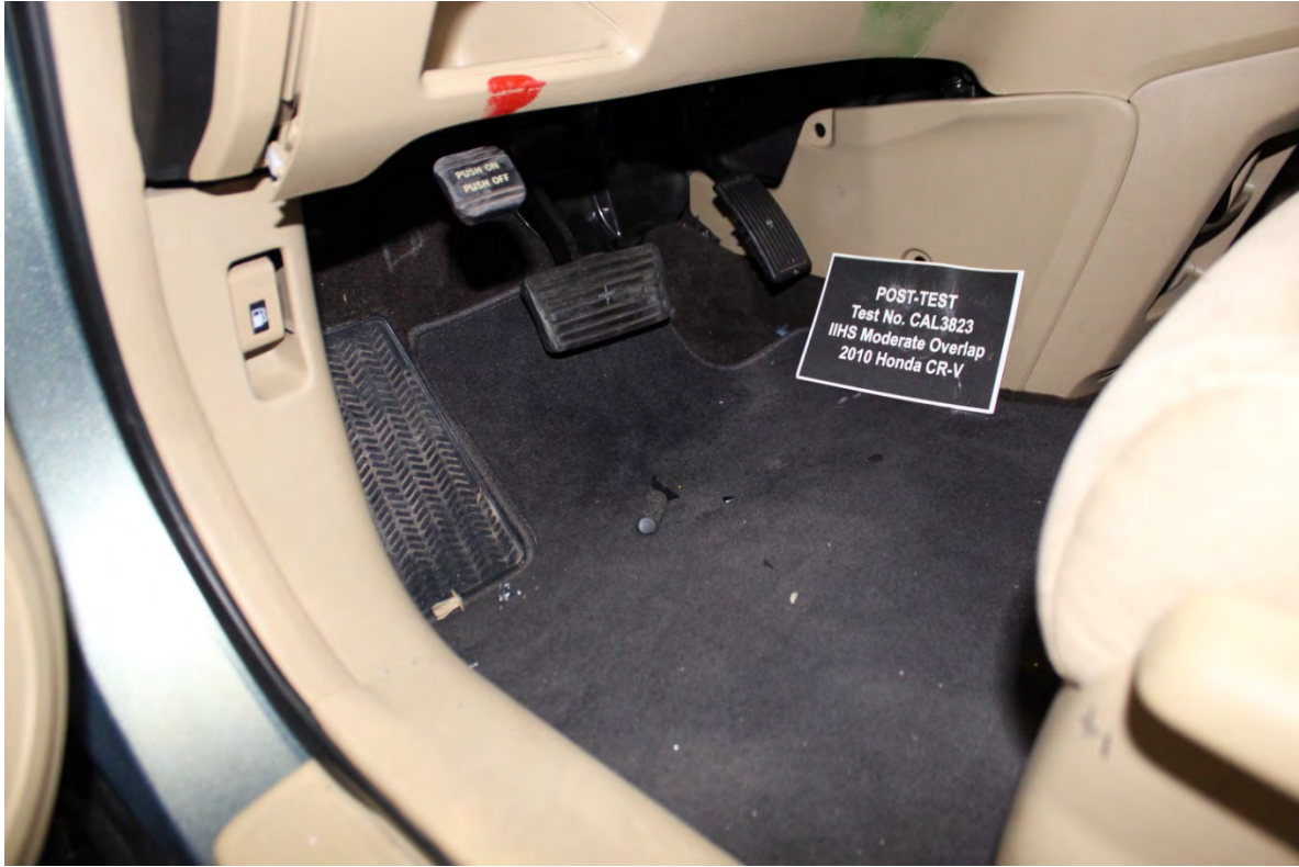
Footwell intrusion and paint mark from dummy's body after displacing the dummy
