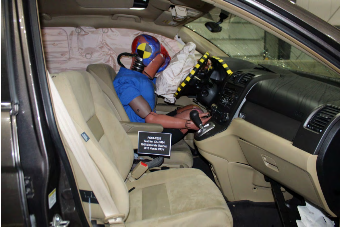
Passenger side view of driver seat after the crash test
