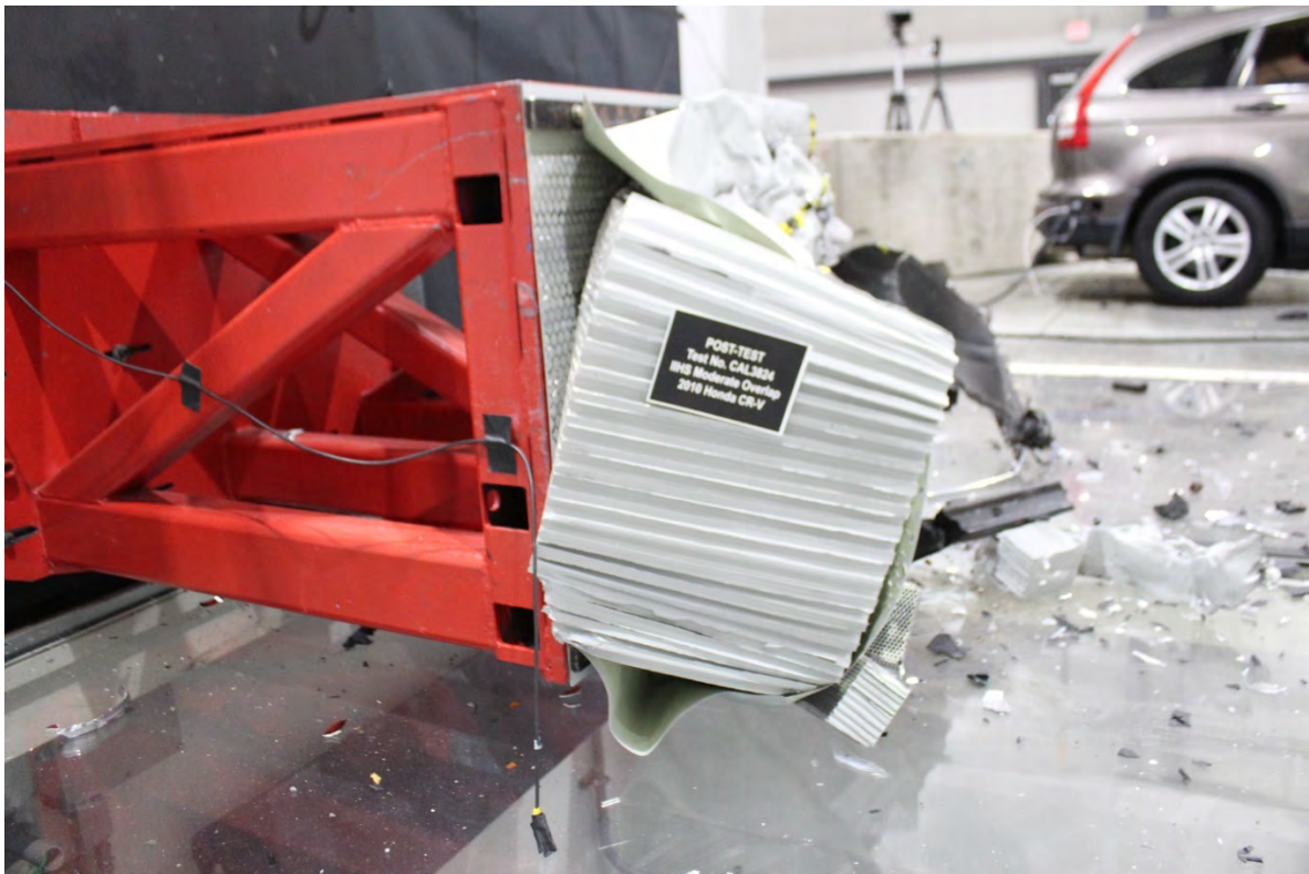
Left side view of deformed barrier
