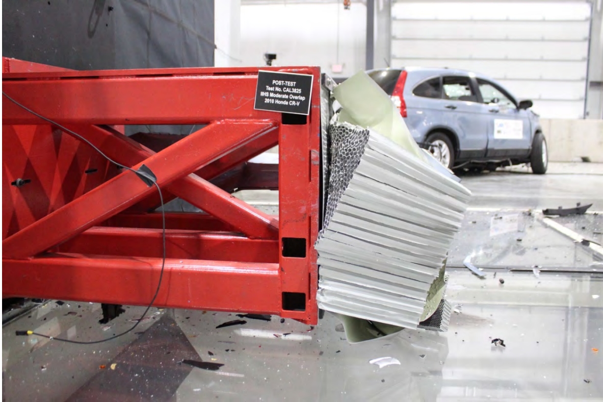
Left side view of deformed barrier
