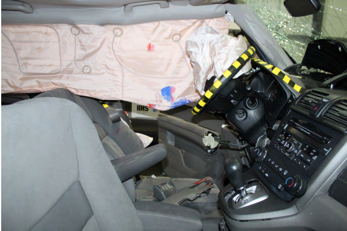
Inside view of vehicle with deployed side airbag and significant intrusion
