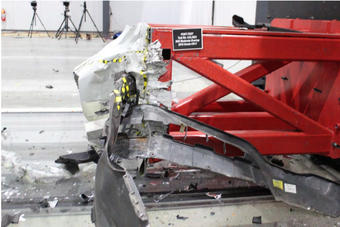
Right side view of deformed barrier
