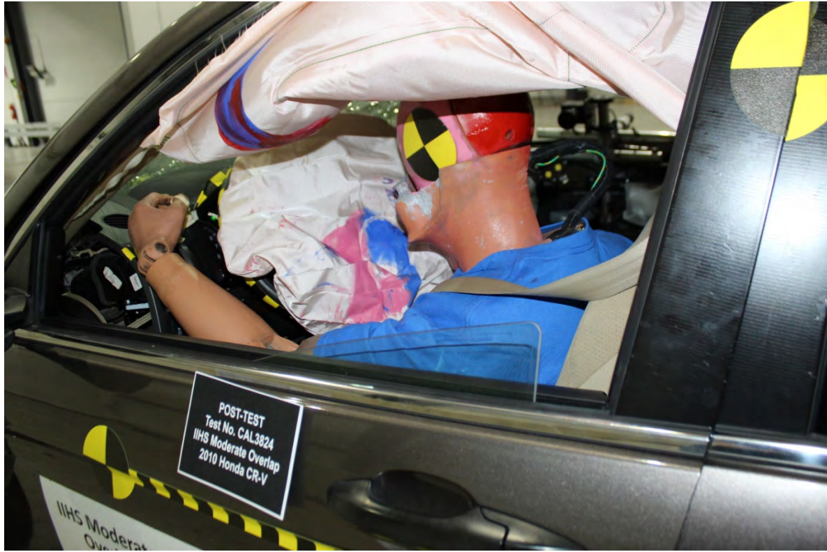
Deployed airbag with paint mark from the dummy's head
