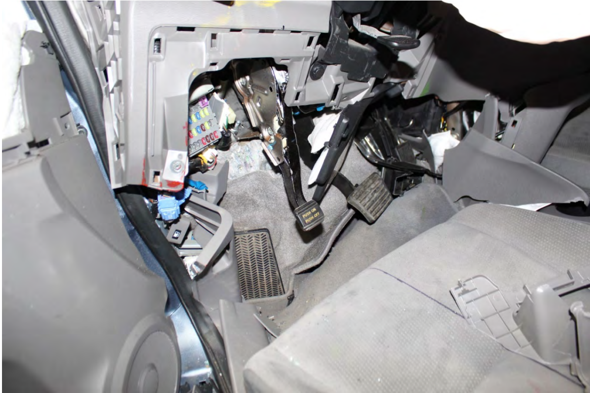
Significant footwell intrusion
