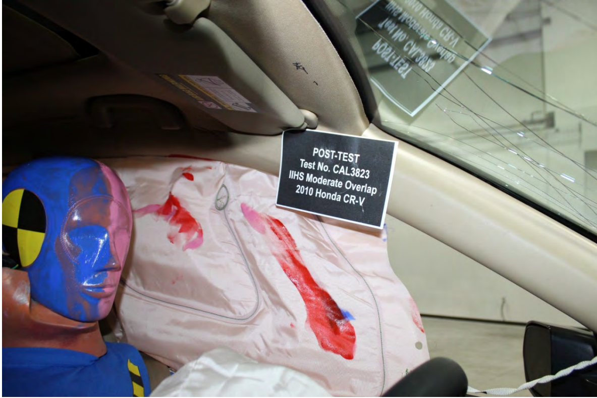
Deployed curtain airbag with paint mark applied to the dummy's head before test
