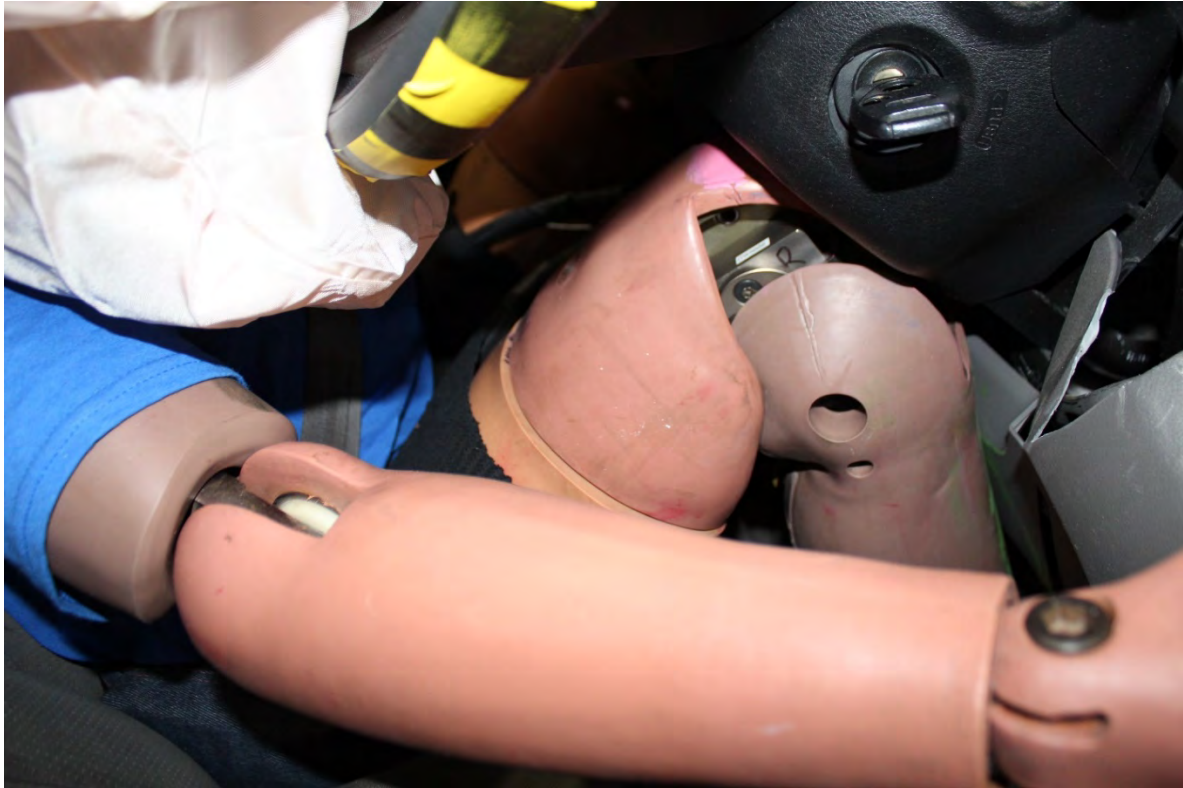
Dummy's right knee contacting the steering wheel column
