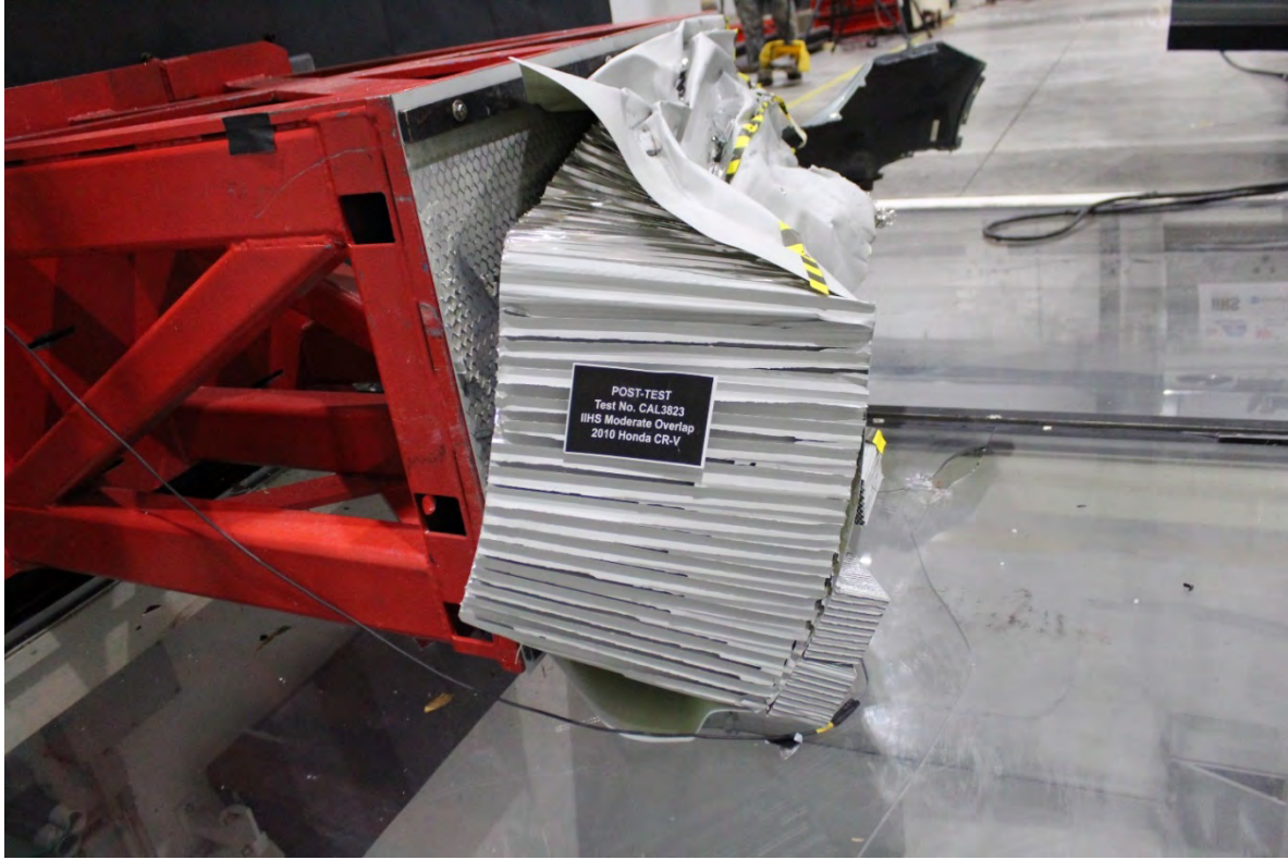
Left side view of deformed barrier
