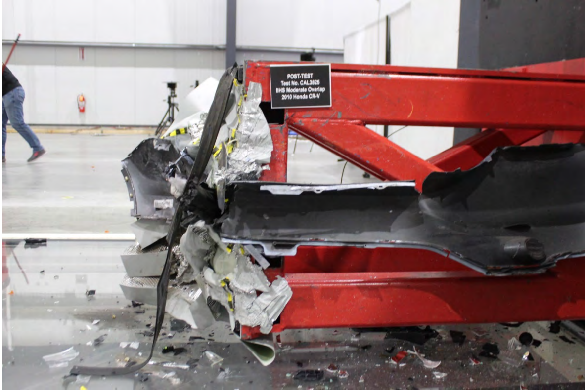
Right side view of deformed barrier
