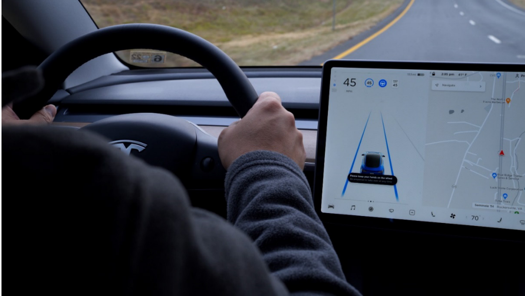
Figure 2. Photo of Tesla Model 3 interior showing the combined instrument panel and center stack display next to the steering wheel.
