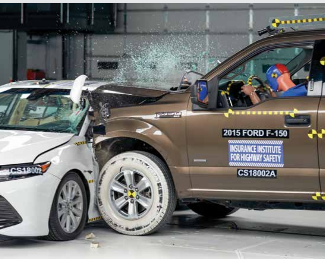
This 37 mph crash of a 2015 Ford F-150 into a 2018 Toyota Camry is part of a series of research tests investigating how the IIHS side crash evaluation might be improved.
