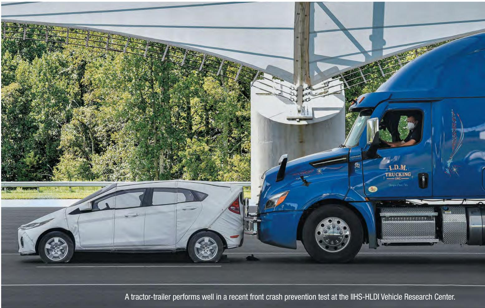
A tractor-trailer performs well in a recent front crash prevention test at the IIHS-HLDI Vehicle Research Center.
